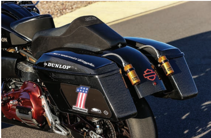
Remote Reservoir Screamin' Eagle by Öhlins 36mm dual shocks were developed by the Swedish suspension manufacturer with extensive testing and input from Kyle Wyman and his crew. Photo by Brian J. Nelson.
