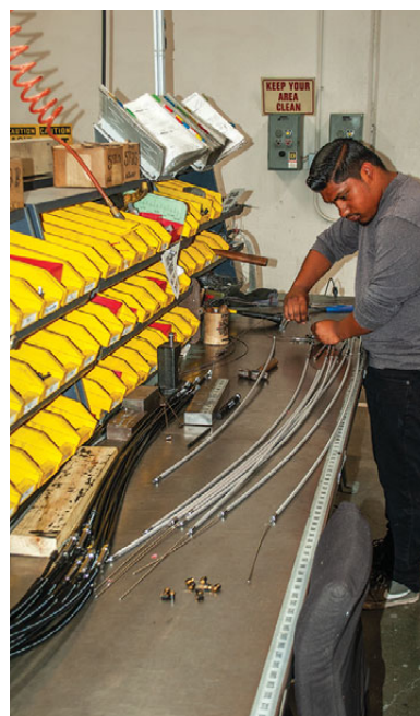
(Above Left) The blue saw and the green press above cut and stamp clutch plate blanks from aluminum and steel, respectively. (Above Right) A worker assembles control cables. (Below) A cam-driven screw-type lathe carves brass fittings for control cables and hydraulic lines.
