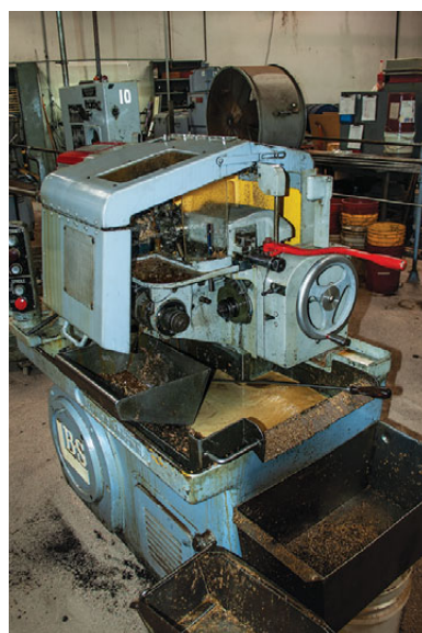
(Above Left) The blue saw and the green press above cut and stamp clutch plate blanks from aluminum and steel, respectively. (Above Right) A worker assembles control cables. (Below) A cam-driven screw-type lathe carves brass fittings for control cables and hydraulic lines.
