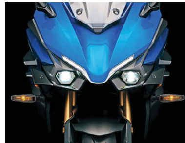
The nose of the GSX-S1000GT+, showing dual LED headlights; aero includes relatively small winglets.
