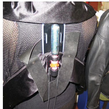
(Above) Cutaway Vanson street jacket equipped with the Vanson CO 2 airbag system. Stretch panels make room for airbag inflation.
